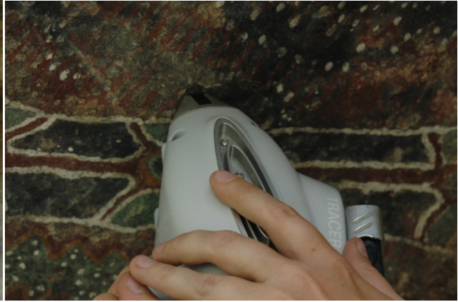
Figure 18. Portable XRF in use on in situ rock art Figure 19. Close up of Portable XRF device in use
